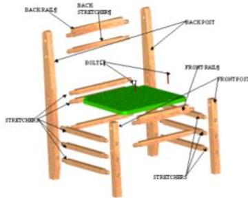
Figure 1: Exploded view of 14" chair components
