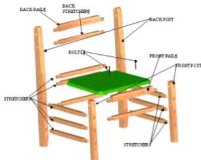
Figure 1: Exploded view of 14" chair, showing all components
