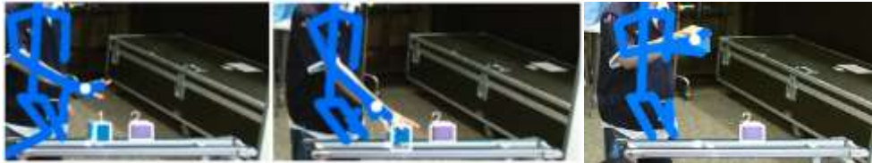
Fig. 14. Using the skeleton data (specifically hand position) and the position of the object to infer tasks such as approach and transport.
