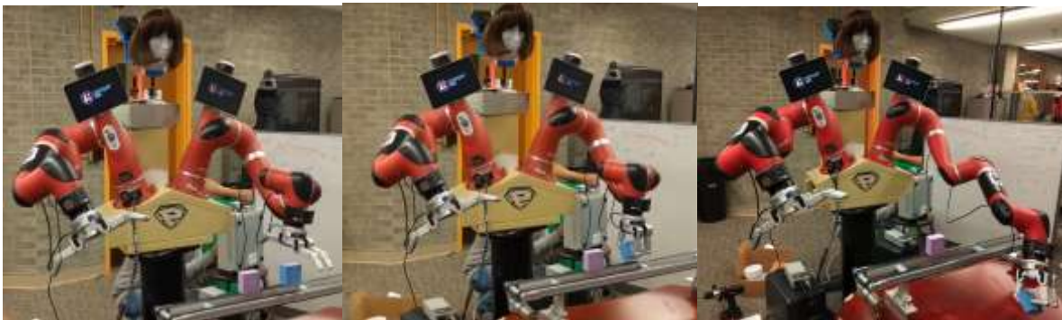
Fig. 15. Pick and place task performed by Super Baxter with visual servoing
