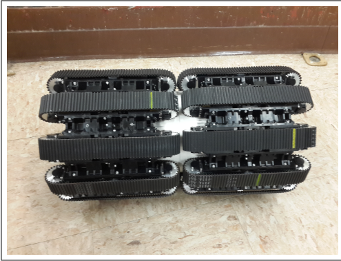
Fig. 5. The 2-D tread module configured as a holonomic differential drive platform.
