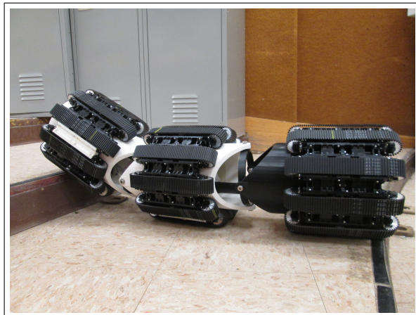
Fig. 1. The 2-D tread module assembled into the MOTHERSHIP hybrid serpentine configuration.
