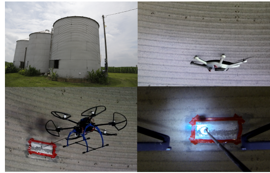
Fig. 4. flight tests in a silo, including outside look of the silo, CyPhy LVL 1 flying inside doing inspection, Dexterous Hexrotor taking samples, first person view during sampling.
