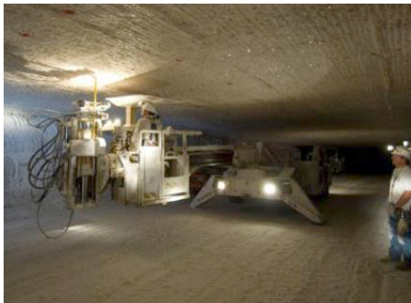
Bolting in uncontaminated areas, a critical periodic maintenance step, resumed in November, 2014.
