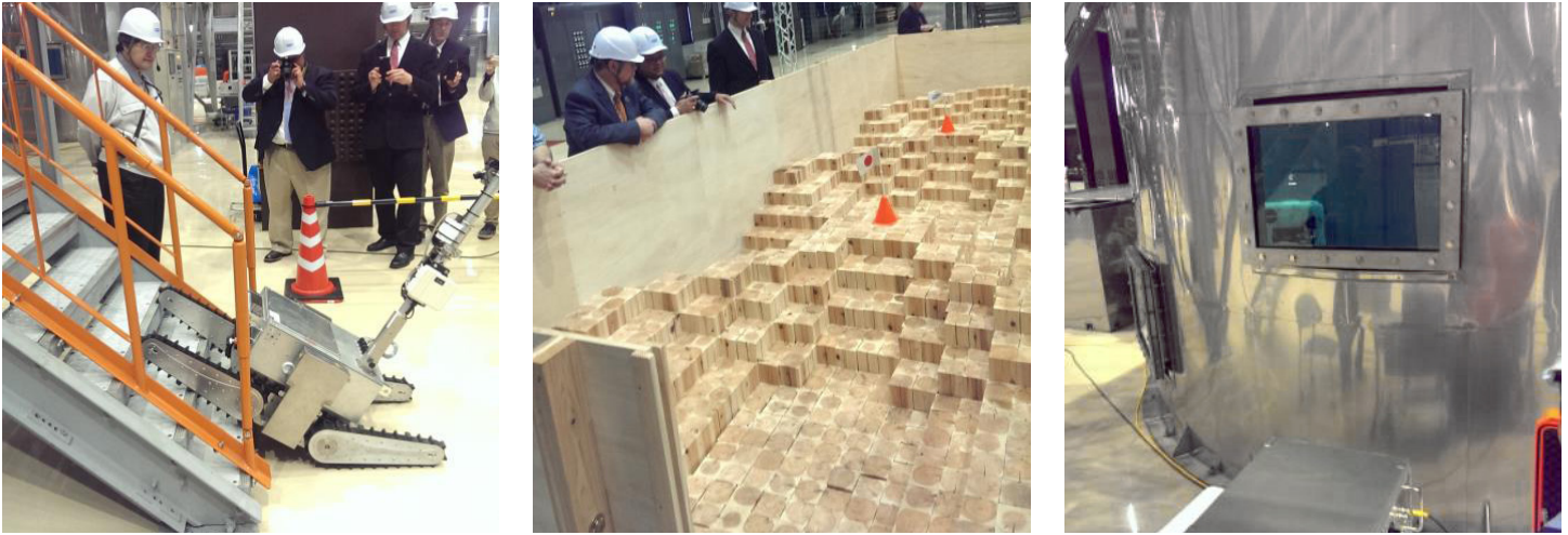
The Naraha Test Facility has a customizable stair system to model stairs of different sizes and formats (left).
