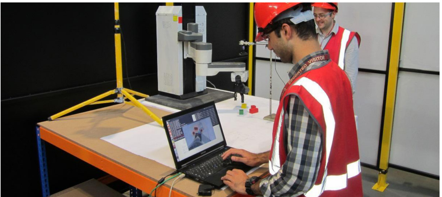
Workers at NNL set up a lab test with a mock pick-and-place operation.
