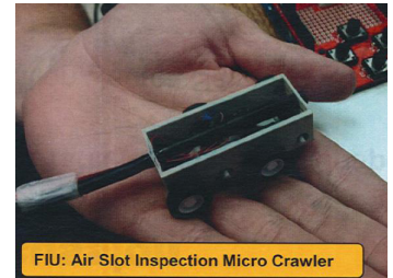
Examples of miniaturized systems under development for inspecting air slots and other extremely small spaces.
