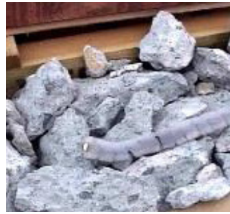
Tohoku's Active Scope Camera (ASC) on a pile of rocks in the lab (left) and the operator console with PlayStation controller (right).
