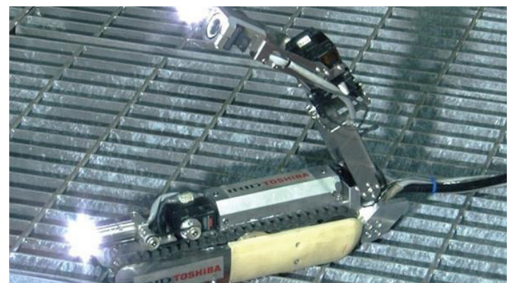
Rod Rimando, DOE, at Toshiba with a copy of the shape-changing "scorpion" robot that plans to enter the containment vessel (left). Posed image of the robot on a grate (right).
