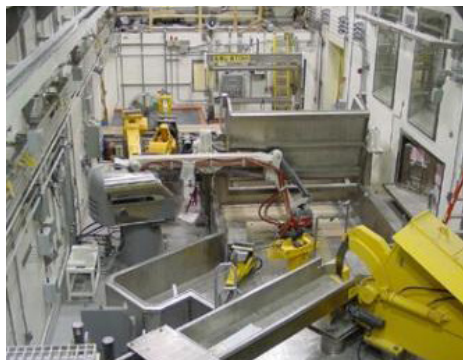
A work cell containing robot arms and conveyors is used to sort mixed waste.
