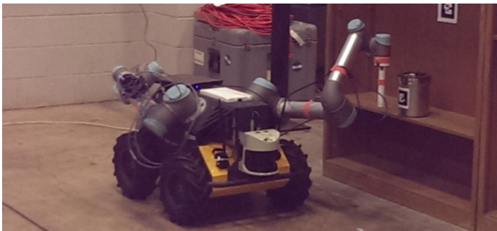
A bi-manual mobile robot for inspecting radiological samples in a warehouse environment, left. Another warehouse inspecting robot “sniffs” the floor to look for possible spills and other forms of localized contamination, right. This robot tirelessly searches the entire floor and maps evidence of contamination for future comparisons.
