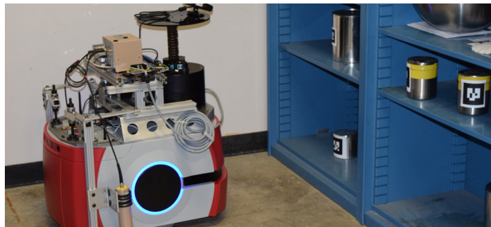
A bi-manual mobile robot for inspecting radiological samples in a warehouse environment, left. Another warehouse inspecting robot “sniffs” the floor to look for possible spills and other forms of localized contamination, right. This robot tirelessly searches the entire floor and maps evidence of contamination for future comparisons.
