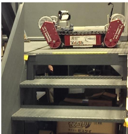
Mock-up tower at Tohoku University rescue robotics facility with Quince robot (left).
