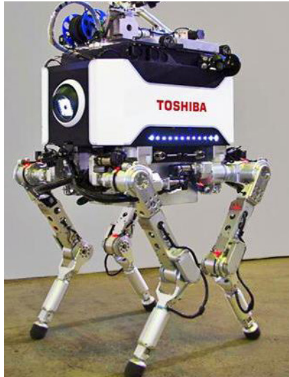
Toshiba quadruped robot that can climb stairs and carries a remote, tethered robot for inspection. An underwater inspection robot, far right, inspects inside the reactor vessel.
