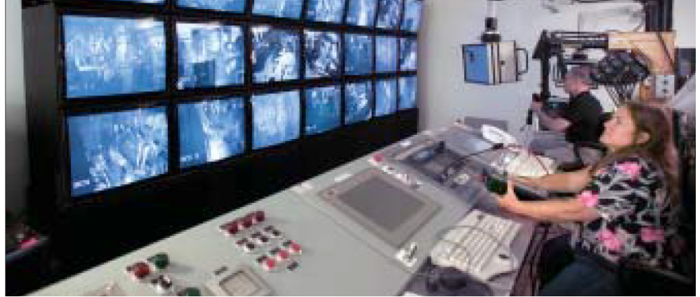
Left: A teleoperated dual-arm servomanipulator is used for dexterous remote handling operations in hot cell work areas at the Spallation Neutron Source at a modern DOE facility at Oak Ridge National laboratory. Right: A remote operator controls the dual-arm servomanipulator from a control room equipped with a multi-camera viewing system.
