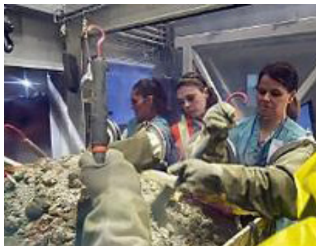
Human workers process waste through glovebox portals.
