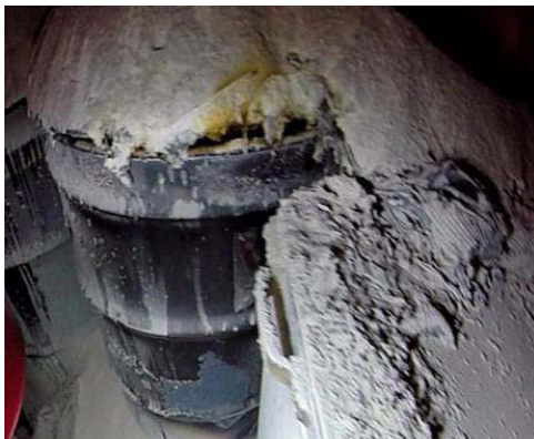
An image of the ruptured canister that released radiation on February 14, 2014.
