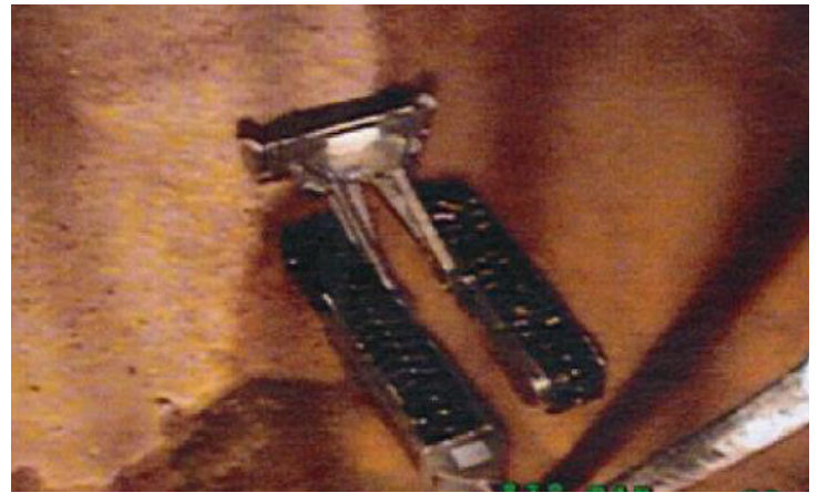
The FoldTrack robotic vehicle for cleaning inside of tanks with limited access risers.
