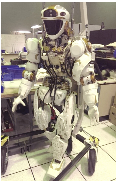
Valkyrie is the latest NASA/JSC humanoid that competed in the DARPA Robotics Challenge. Right, the RoboGlove, a "power glove" for human augmentation to reduce fatigue, is derived from Valkyrie. (right image courtesy NASA)
