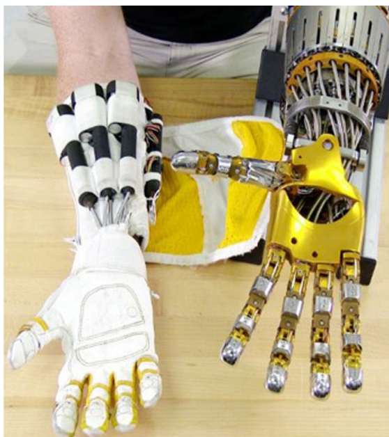
Valkyrie is the latest NASA/JSC humanoid that competed in the DARPA Robotics Challenge. Right, the RoboGlove, a "power glove" for human augmentation to reduce fatigue, is derived from Valkyrie. (right image courtesy NASA)
