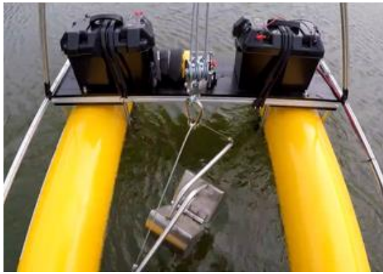
(a) Van Veen grab sampler from the USV
