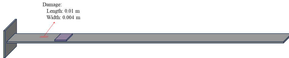
Figure 6-5. Illustration of small-sized damage in the host structure.
