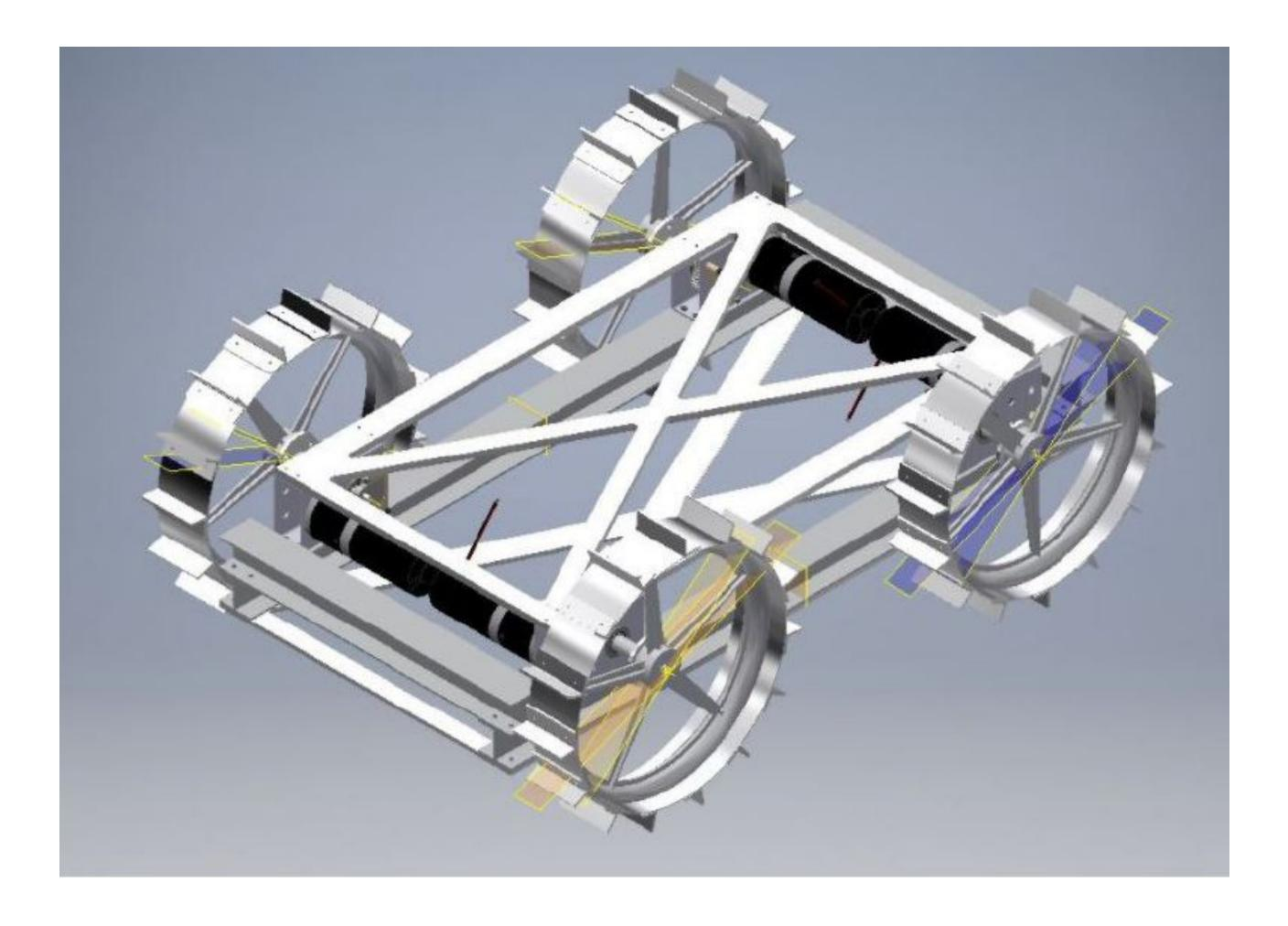
Post testing analysis shows the chassis performed as expected. Its light weight and ease of manufacturing benefitted maintenance greatly. Further improvements will include better power management and improved layout for the mining platform.
