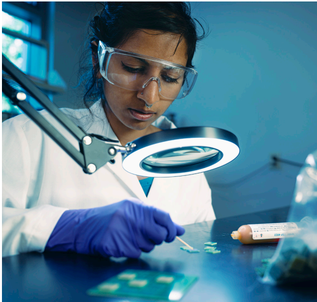
A student places solder balls on a BGA test board in the electrical materials lab. (Purdue University/Charles Jischke)
