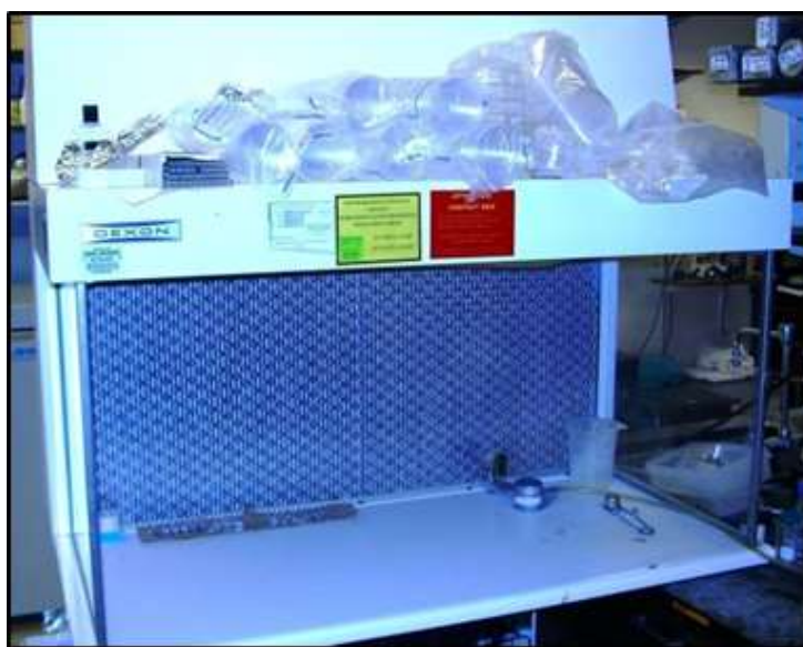
Figure 4.4 – Laminar Flow Clean Bench
