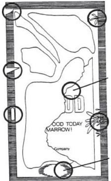
Folded over wrinkles cause by one side being longer than the other
