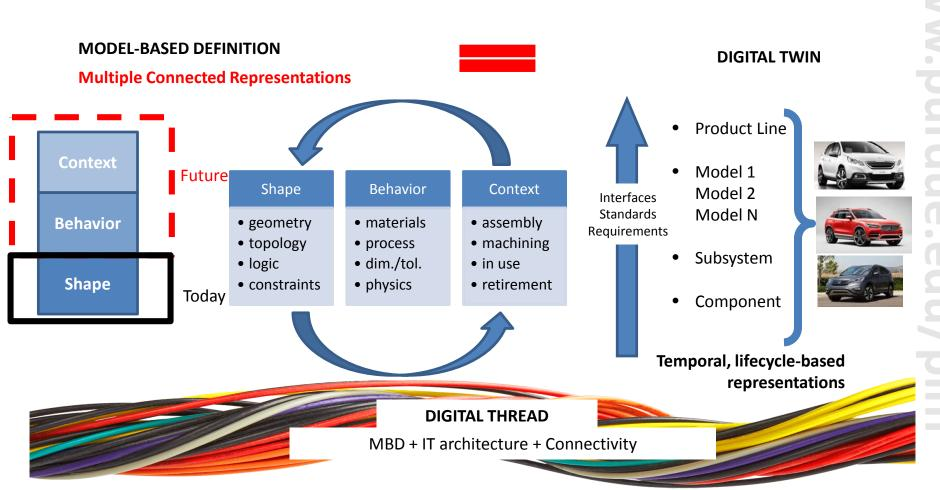
By comparing digital product data to the physical performance of the object, variation can be tracked and used to inform design of next-generation products, develop predictive modeling and validation schemes for products, and to diagnose and solve problems that occur.
