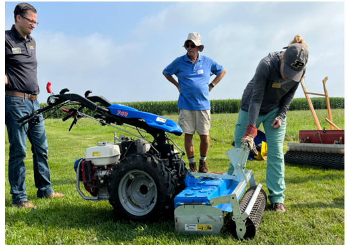
Ashley Adair explains operation of power harrow attached to BCS walk-behind tractor.
