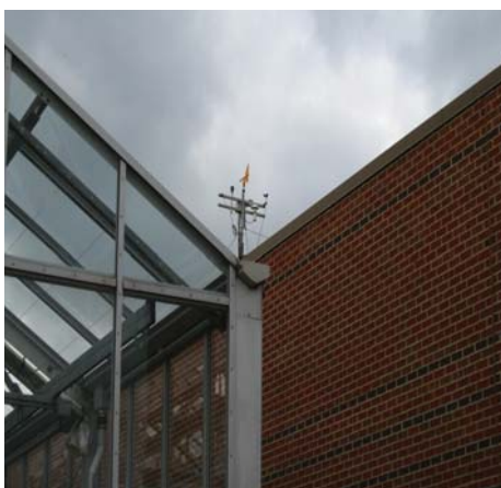
Figure 2. Weather stations can record temperature, humidity, wind, precipitation, and light level to assist in greenhouse environmental control.
