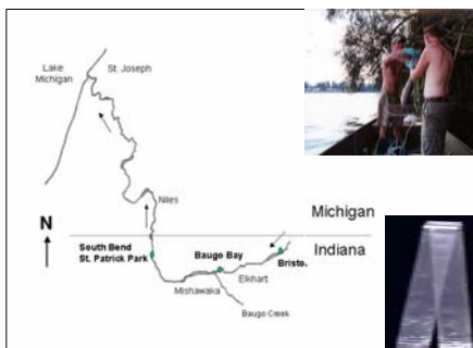
Figure 1. Map of St. Joseph River, IN, U.S.A. showing location of study sites; (1) Bristol; (2) Baugo Bay; (3) d/s South Bend St. Patrick Park. (inserts) Students deploying SPMDs in wire cages. An SPMD.
