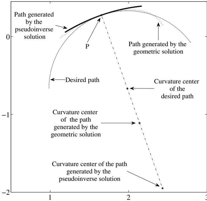
**Fig. 2** The planar 3R mechanism is required to track the circular arc passing through point  $P$ . The dashed curve is the geometric tracking solution, and the solid curve is the pseudoinverse tracking solution. The curvature centers of the three paths are shown.
