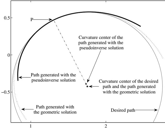
**Fig. 1** The planar 3R mechanism is required to track the circular arc passing through point  $P$ . The dashed curve is the geometric tracking solution. The solid curve is the pseudoinverse tracking solution. Curvature centers for the three paths are shown. Only the curvature centers of the desired path and the path generated with the geometric solution match.
