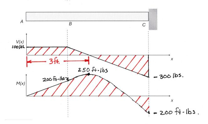
d) Indicate the location on the beam which has a point in pure bending by stating its location from the left end of the beam. For the point experiencing pure bending, find the value of the maximum tensile normal stress and the location on the cross section where it occurs. (6 pts)
