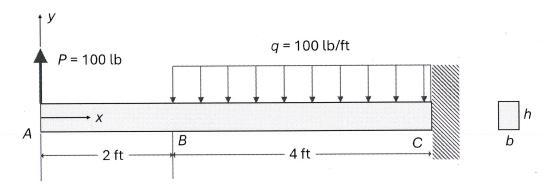
**FIND:** a) Draw the overall free body diagram on the artwork provided below (**2 pts**). Use the single equivalent force for the uniform distributed load. Determine the reactions at the fixed end *C* and write them in the box below. (**5 pts**)
