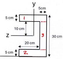
$$T_{Z} = T_{1} + Ad_{1}^{2} + T_{2} + A_{2}d_{2}^{2} + T_{3} + A_{3}d_{3}^{2}$$
