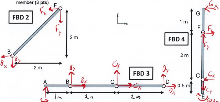
d) Solve for the internal forces at joints B and C on member ABC. Express the resultant forces in vector form. (8 pts)
