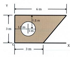
$$A_{ToT}(\chi_c) = A_1 \times c_1 + A_2 \times c_2 + A_3 \times c_3$$
