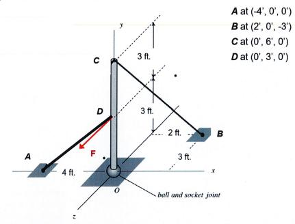
a) Complete the free body diagram of the pole using the artwork below by adding FBD components at **point O**. (**9 pts**)
