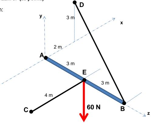
A 60 Newton load is applied to a massless rod.
