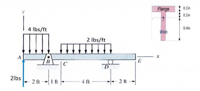
FIND: a) Draw the free body diagram (1 pt) of the beam ABCDE and calculate the reaction forces at the supports in vector form. (6 pts).
