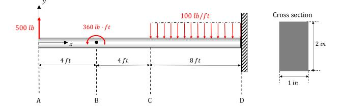
The cantilever beam is subjected to the loading condition as shown below.
