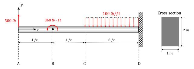
a) Draw the Free-Body Diagram of the beam and determine the reactions at the wall. Write your answer in the given box.
