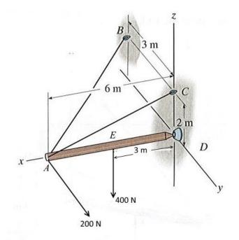
b) Express the tension in cables  $\overline{T}_{AB}$  and  $\overline{T}_{AC}$  in terms of their unknown magnitudes and their known unit vectors. Write the vectors in decimal form (not as fractions). (4 pts)
