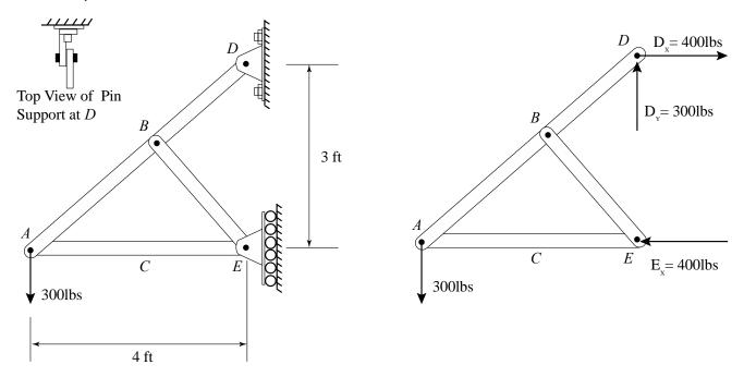
i) Determine the average shear stress and shear strain for pin D.
