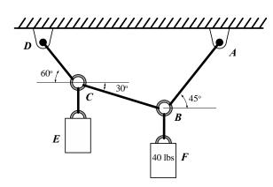
**Problem 1A. (5 pts.)** The cylinder F weighs 40lbs. and is supported by cables BC and BA. Cables BC and DC also support cylinder E whose weight is not known. Determine the magnitude of the tension in cables BC and BA.
