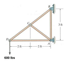
$F_{CD} = T$  or C (3pts) Zero-Force Members = **1(c)** One the members provided, sketch the free body diagram of the two member frame. Determine the force  $F_{AB}$  acting on member BC in vector form.
