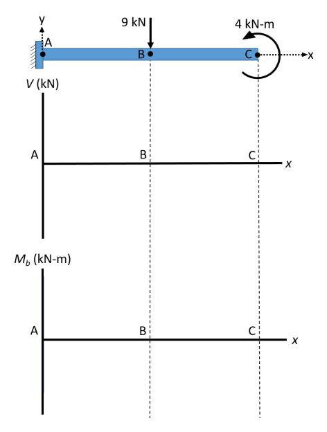
4C. Over what section is the beam in pure bending (1 pt)?
