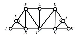
d) Using the method of sections, sketch an appropriate free-body diagram, determine the magnitudes of the forces in members CH and CD, and identify whether each member is in tension, zero, or compression (6 pts):
