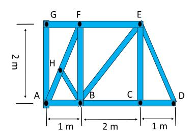
b) Determine the support reactions at A and G. The signs of the reaction forces should be consistent with your free body diagram. (3 pts)
