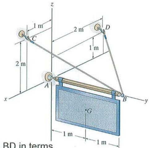
$$b) \bar{T}_{BC} = T_{BC} \left( \bar{u}_{BC} \right)$$
