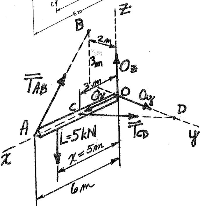
$$\sum M_O = 0 = (\vec{r}_{OA} \times \vec{T}_{AB}) + (\vec{r}_{OC} \times \vec{T}_{CD}) + (\vec{r}_{OL} \times \vec{L})$$
