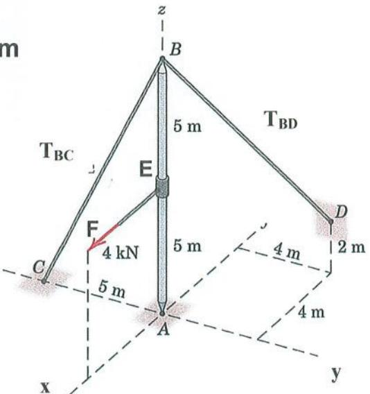
$$b) \quad \overline{T}_{BC} = T_{BC} \left( \overline{u}_{BC} \right) \\ = T_{BC} \frac{(-5\overline{j} - 10\overline{k})}{\sqrt{(-5)^2 + (-10)^2}}$$
