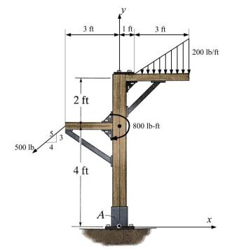
b) Draw the free body diagram of the system, list all applied and reaction forces and moments, replace the triangular distributed load with a single equivalent load and mark its location. (3 pts)
