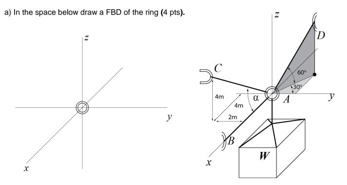
b) Resolve the tension in ropes AB, AC and AD in Cartesian vector form.
