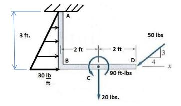
c) Determine the reactions at the fixed support A required to hold bar ABCD in static equilibrium. (10 pts)
