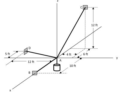
**c)** Using your equations of static equilibrium, determine the magnitude of the forces in cables AB, AC, and AD. (10 pts)
