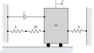
a) What is the undamped natural frequency  $\omega_n$ ?
