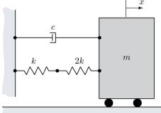
a) What is the undamped natural frequency  $\omega_n$ ?
