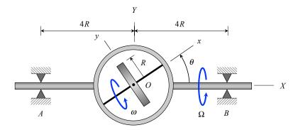
A shaft is supported by bearings A and B, with the shaft rigidly supporting a ring. The shaft is rotating with a constant rate of  $\Omega$ . A thin disk of radius R and mass m is attached to a second shaft that is rotating with a constant rate of  $\omega$  on bearings in the ring, as shown. Ignore all mass in the system except for that of the disk. For the position shown, determine the reactions on the shaft due to the bearings at A and B.
