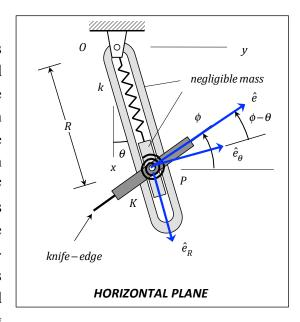
is unstretched when  $\phi = 0$ , and the spring between O and P is unstretched when  $R = R_0$ .
