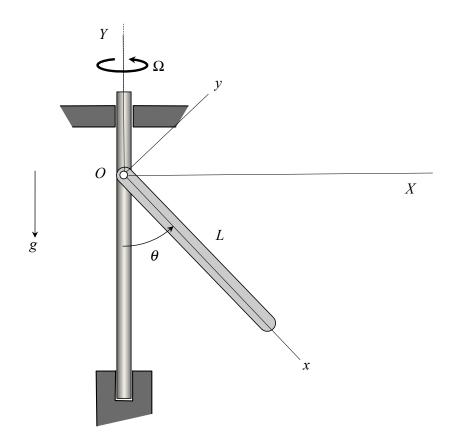
A thin, homogeneous bar of mass m is pinned to a vertical shaft at end O. The vertical shaft is allowed to rotate freely. The bar is released with initial conditions of:  $\theta(0)=10^{\circ}$ ,  $\dot{\theta}(0)=4$  rad / sec and  $\Omega(0)=10$  rad / sec. Using an energy approach, determine the total angular velocity of the bar when  $\theta=90^{\circ}$ . Use L=2m.
