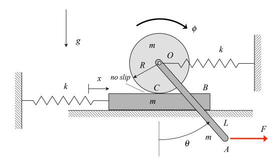
Consider the system shown above made up of a homogeneous disk, a thin homogeneous bar OA and a block. The surface on which the block slides is smooth; however, the disk rolls without slipping on the block. The springs are unstretched when  $x = \phi = 0$ . Using Lagrange's equation, develop the equations of motion for the system.
