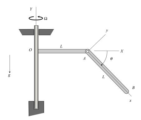
A thin homogeneous bar, AB, of mass m, is pinned to arm OA. Arm OA is welded to the vertical shaft, as shown. The vertical shaft is constrained to be rotating with a constant speed of  $\Omega$ . Using Lagrange's equations, the differential equation of motion of arm AB in terms of the angle  $\theta$ .
