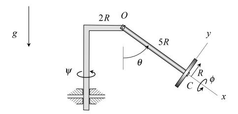
A thin disk of mass m and radius R is allowed to rotate about end C of shaft OC with constant angular speed of  $\dot{\phi}$ , with the orientation of shaft relative to the vertical being  $\theta$ . Shaft OC has a mass of m. The rotation of the L-shaped shaft is rotating is represented by the angle  $\psi$ . Assume that OC is aligned with the symmetry axis of the disk. Using Lagrange's equations, develop the equations of motion for the system.
