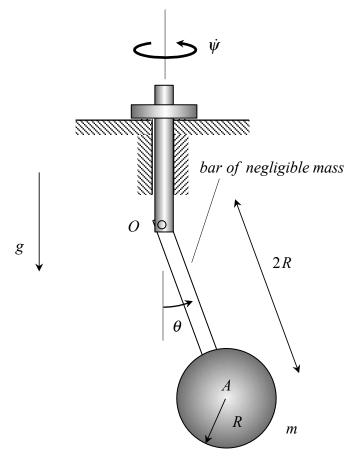
A homogeneous sphere of mass m and radius R is attached to a bar having negligible mass. This bar is pinned to a vertical shaft at end O, with the shaft rotating about its fixed axis with a constant rate of  $\dot{\psi}$ . Let  $\theta$  represent the angle between OA and a fixed vertical line.
