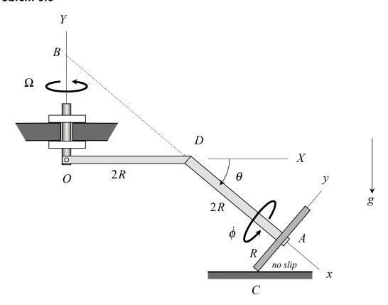
A thin disk of mass m rolls without slipping on a flat, horizontal surface as it freely rotates about the bent arm, as shown, with the arm having negligible mass. The arm, in turn, is pinned to a shaft at O with the shaft being constrained to rotate about its vertical axis with a constant speed of  $\Omega$ . Determine the normal force acting on the disk by the horizontal surface on which it rolls.
