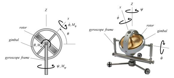
Consider the rotor of the above gyroscope to be a thin disk of mass m and radius R. Ignore the mass of the gimbal and gyroscope frame. The center of mass of the disk lies on the fixed Z-axis. At some instant in time when the gyroscope has three non-zero rotation rates  $\dot{\phi}$ ,  $\dot{\theta}$  and  $\dot{\psi}$ , a torque of  $M_{\psi}$  is applied to the frame. Determine  $\ddot{\theta}$  as a result of this applied torque.
