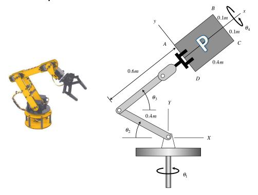
Consider the robotic arm shown above holding a rectangular sign ABCD in its end effector. Let the XYZ axes be fixed in space, and the xyz axes attached to the sign. When  $\theta_1 = \theta_3 = \theta_4 = 0$ , the xyz and XYZ axes are aligned. With  $\theta_2 = 90^\circ$  held fixed, consider the three rotations through which the robotic arms is taken:
