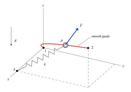
Particle P, having a mass of m = 2kg, is able to slide on a smooth guide, with the shape of the guide described by the following Cartesian coordinates (in cm):
