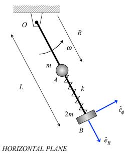
Particle B (of mass 2m) is attached to rigid rod OB with the rod having negligible mass and a length L. Particle A (of mass m) is allowed to slide along the smooth rod OB with a spring of stiffness k connecting A and B. The spring has an unstretched length of L/2. The system is given a set of initial conditions of  $\omega = \omega_1$ ,  $R = R_1 = L/2$  and  $\dot{R}_1 = 0$ . Determine the polar coordinates for the velocities of A and B when  $R = R_2 = 3L/4$ .
