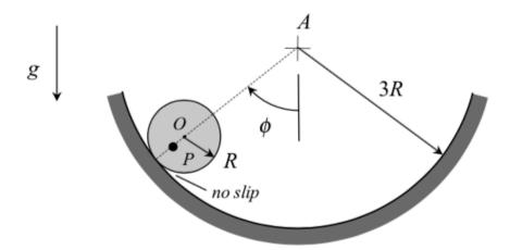
Particle P (having a mass of m) is embedded in a disk (having negligible mass and outer radius R) rolls within slipping on the inner surface of circular bowl, with this inner surface of the bowl has a radius of 3R. P is located at a radial distance of R/4 from the disk's center O. Let  $\phi$  measure the angle between the vertical and the position of O. The system is released from rest with  $\phi = 60^{\circ}$  and with P on the radial line OA.
