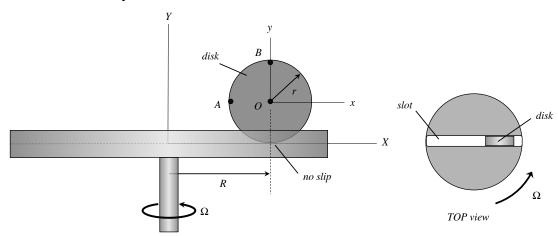
A turntable rotates about a fixed axis with a constant rotation rate  $\Omega$ . A circular disk, having an outer radius of r, rolls without slipping within a radial slot cut in the top surface of the turntable in such a way that  $\dot{R} = constant$ , where R is the radial distance from the turntable's rotation axis and the center O of the disk.
