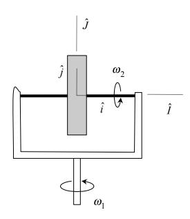
Given: Shaft BD rotates about a fixed axis with a constant rate of  $\omega_1$ . Shaft OA is rigidly attached to shaft BD with OA being perpendicular to BD. A disk rotates about shaft OA with a constant rate of  $\omega_2$  relative to OA.
