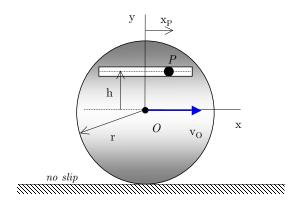
Given: The disk of radius R rolls without slipping on a horizontal surface with the speed and acceleration of the disk center O given by  $v_O$  and  $a_O$ , respectively. A particle P slides within a semi-circular slot cut in the disk with P moving with a speed of u relative to the disk and a rate of change of speed of  $\dot{u}$  relative to the disk. The radius of the slot is R.
