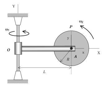
Given: Arm OC rotates about the fixed Y-axis at a constant rate  $\Omega$ . The disk at C, having a radius of R, is able to rotate about arm OC and rolls without slipping on a fixed horizontal surface. Let the xyz axes be attached to the disk.
