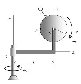
Given: The disk of a gyroscope rotates about its own axis at a constant rate of  $\omega_2 = 600$  rev/min. The gimbal support is rotating at a constant rate of  $\omega_1 = 10$  rad/s about a fixed vertical axis. The observer and the xyz axes are attached to the disk. The XYZ axes are fixed in space.
