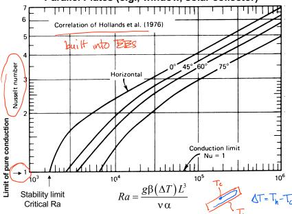
L = plate spacing;  $\beta$ =1/ $T_{avg}$  (for air);  $\Delta T$  is temperature difference between surfaces of parallel places; use 75° curve for vertical plates
