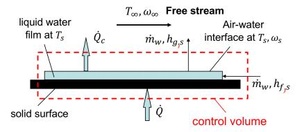
where  $\dot{Q}_c$  is convective (sensible) heat transfer rate from surface to air,  $\dot{m}_w$  is the water mass flow rate (water vapor from surface due to mass transfer and liquid water make up to surface),  $\dot{Q}$  is the total heat transfer rate to the surface to balance energy flows
