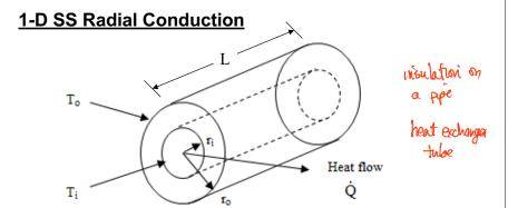
From Fourier's law, the heat transfer rate at any cross-section in the radial direction is
