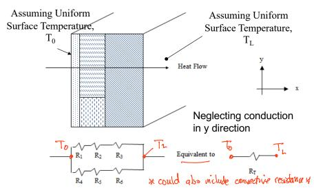
Add resistances (R's) that are in series and add conductances (1/R) that are in parallel to determine overall resistance to heat transfer
