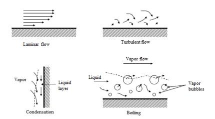
Heat transfer is enhanced through turbulence and two-phase heat transfer
