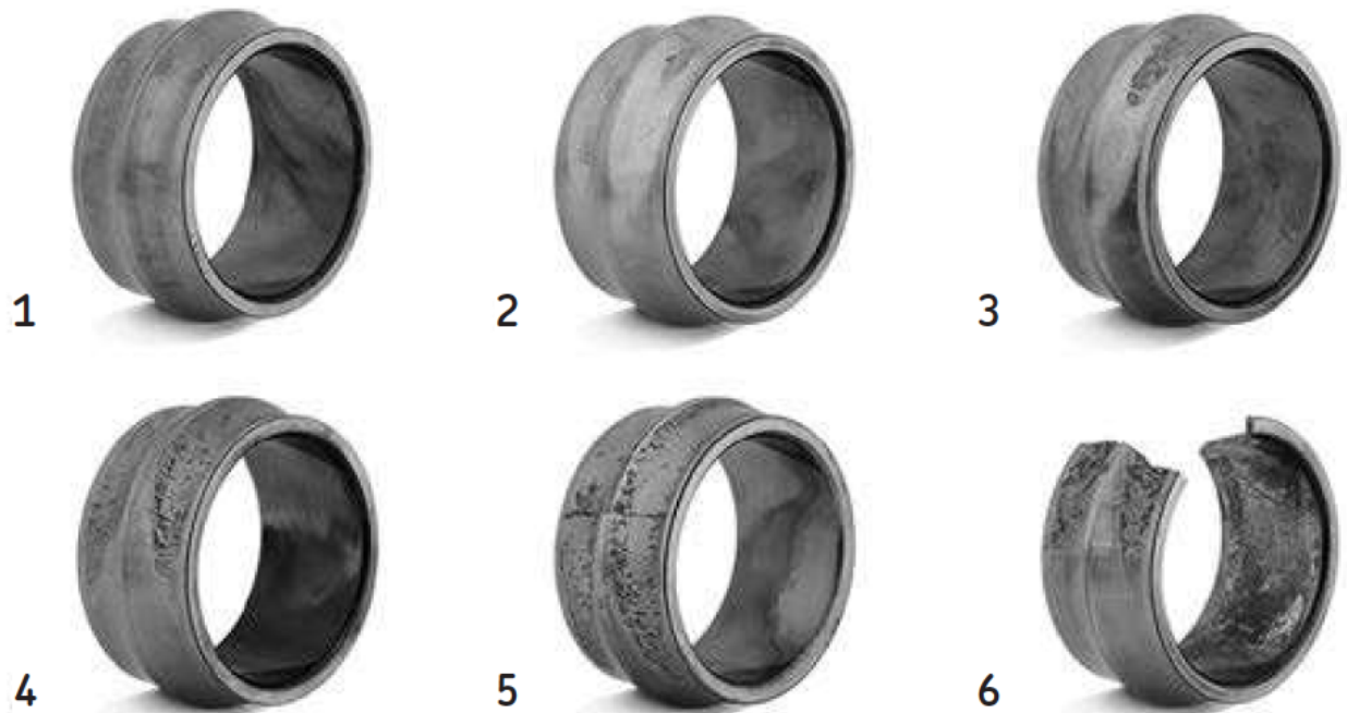
Figure 22: The progression of surface fatigue failure shown on the inner raceway of a rolling element bearing.
