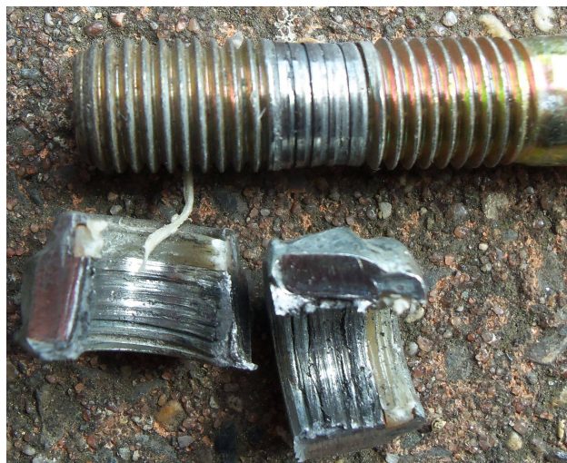
Figure 54: A bolt with stripped threads.
