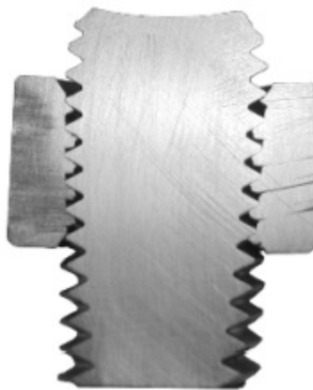
Figure 55: All engaged threads do not share the load due to inaccuracies in thread spacing.
