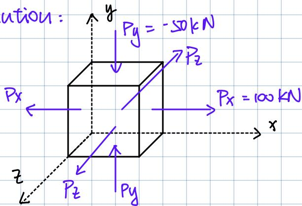
$$\sigma_x = P_x / A_x = \frac{100 \text{ kN}}{200 \text{ mm}^2} = 500 \text{ MPa} \quad ①$$
