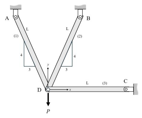
Follow the steps provided below to determine the vertical displacement of pin D:
