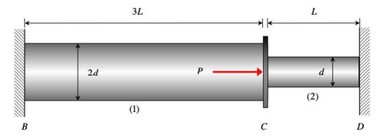
(a) A rod is made up of solid elements (1) and (2) joined by a rigid connector C, with the material of (1) and (2) having the same modulus of elasticity. An axial load P is applied to C with no thermal loads being present. Let  $F_1$  and  $F_2$  represent the axial loads in elements (1) and (2), respectively. Circle the response below which most accurately describes the relative sizes of  $F_1$  and  $F_2$ :
