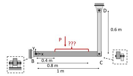
BCD is a shelf that has a double-sided pin at B and a single-sided pin at C. The ultimate stresses of the pins are both 60 MPa. A load of P = 1 kN will be placed on the BC section of the shelf somewhere between 0.4 m and 0.8 m from B.
