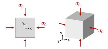
Assume small strains and linear materials properties. For different values of the Poisson's ratio, indicate whether the change in volume ( $\Delta V$ ) and the strain in the z direction ( $\epsilon_z$ ) are >0, =0, or <0.
