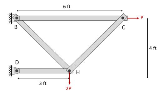
Each of the bars of truss have a cross-sectional area of 1.5 in<sup>2</sup> and an axial failure stress  $\sigma_f = 30 \ ksi$ .
