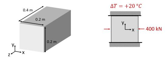
A block of materials has initial dimensions of 0.2, 0.2, and 0.4 m in the x, y, and z directions when no stress is applied. The block is constrained in the y-direction and has a force of 400 kN applied in the x-direction and has no constraint in the z-direction. The temperature of the block is increased by 20 °C ( $\Delta T = 20$  °C). The block is made of epoxy with a Young's modulus of 4 GPa, a Poisson's ratio of 0.45, and a thermal expansion coefficient of 40 x10<sup>-6</sup> °C<sup>-1</sup>.
