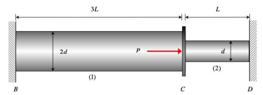
(a) A rod is made up of solid elements (1) and (2) joined by a rigid connector C, with the material of (1) and (2) having the same modulus of elasticity. An axial load P is applied to C with no thermal loads being present. Let  $F_1$  and  $F_2$  represent the axial loads in elements (1) and (2), respectively. Circle the response below which most accurately describes the relative sizes of  $F_1$  and  $F_2$ :
