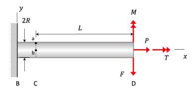
Acting on the cut surface at the wall, we have a shear force F, a bending moment  $M_z = -FL$ , an axial force P and a torque T.
