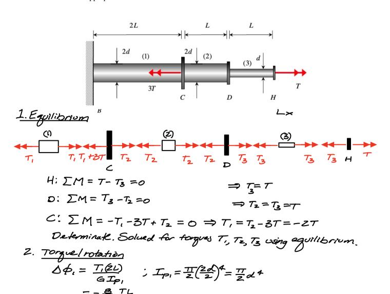
$$D\Phi_{2} = \frac{T_{2}L}{GT_{P2}} ; T_{P2} = T_{P1} = \frac{T_{2}}{2}d^{4}$$
