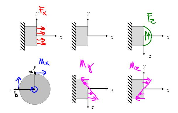
(d) Determine the axial strains  $(\epsilon_x, \epsilon_y, \epsilon_z)$  for the material **point at a** in terms of P, d, and E.
