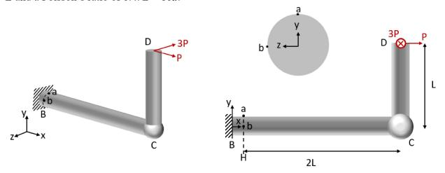
(a) Determine the stresses at points a and b, which are located on cross-section H. a is at the most positive y location of the cross-section and b is at the most positive z location of the cross-section. Indicate the magnitude and sign of the stresses in the table below.
