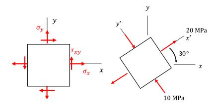
a) Draw the 3D Mohr's circle in the following diagram. Clearly label the three principal stresses and the absolute maximum shear stress.
